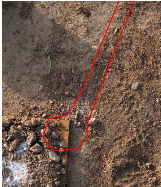
Figure 3. Faint white trail of RDX (outlined in red) dropped by ants. The trail extends from the upper right corner of the RDX panel towards the top right corner of the image.
