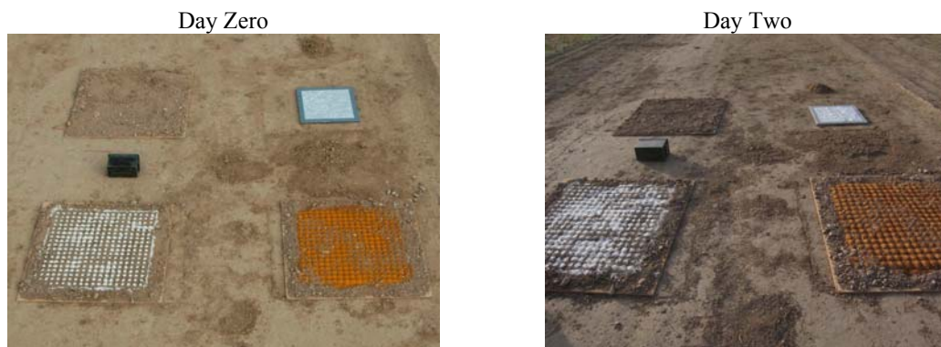
Figure 1. Experiment area showing panels of RDX (white-dotted square, lower left) and TNT (orange-dotted, lower right).
