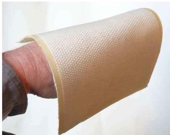
This picture shows an FCC layer without any glass filler. After attaching the balls to the Kevlar with as little silicone as possible and drying it in an oven, I apply a layer of glass filled silicone, levelling it off with the top of the balls. This has no obvious effect on the flexibility.
