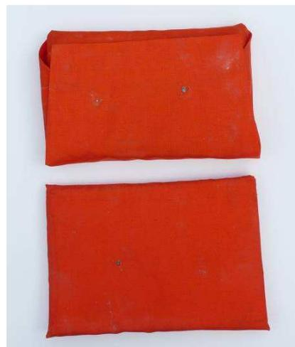
Both shots were stopped inside the FCC. Tiny burn holes were in evidence in the rear of the Ballistic Aramid envelope containing the FCC panel but, although lightly marked, the Kevlar panel behind was not compromised in any way. The burning was indicative of successful kinetic/heat energy transfer.
