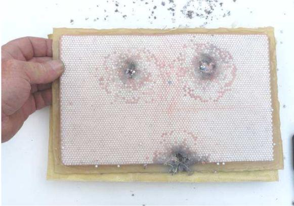
Ceramic balls were displaced over a wide area without breaking.
