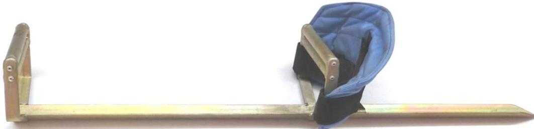
This is the purpose designed MIT excavator. It is not easy to use to scrape spoil away but is easy to use accurately, selecting the point of ground impact with precision. The design minimises the energy required and guarantees that both hands are a distance from the ground while protecting the closest hand. I have used both of these tools and recommend them, but I would not use a short bayonet as a pick-scraper afterwards.
