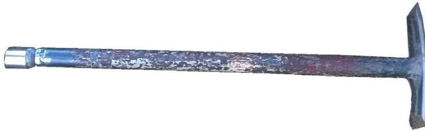
This purpose designed Croatian mini-pick is good, cheap and simple. Made locally, the lump on the end is a neodymium magnet. The pick is used before a bayonet and its flat cutting face can also double as a scraper.
