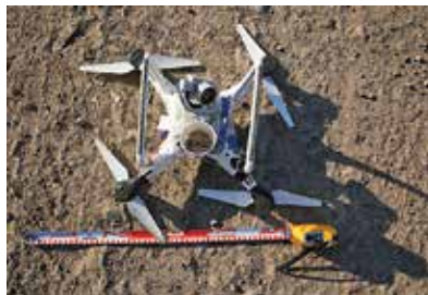
Images 6-8. This commercially available SUA has been adapted to carry and release the small multi-purpose bombs shown. The bombs were manufactured in an ISIS factory.
