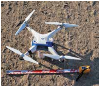
Images 6-8. This commercially available SUA has been adapted to carry and release the small multi-purpose bombs shown. The bombs were manufactured in an ISIS factory.
