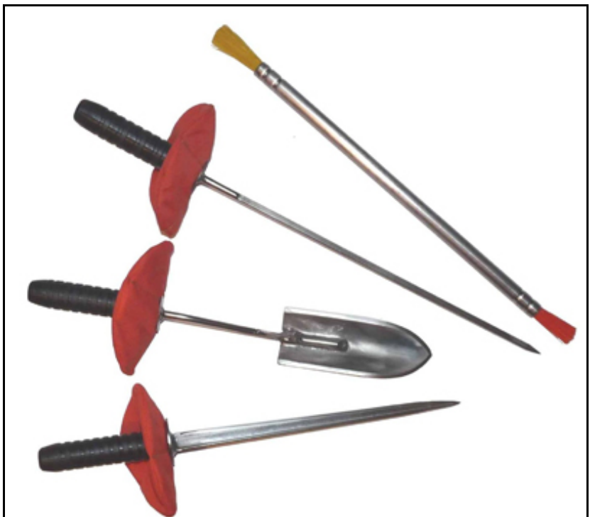
Figure 5. Widely used around the world, the deminer's blast-resistant toolkit was developed with NVESD support in 2000.
