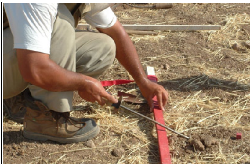
Figure 6. A deminer loosening ground with a prodder in Iraq.
