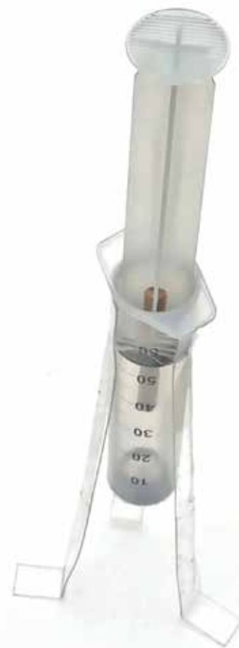
An improvised and low-cost disruptor body with all of the variable control features of those used in our tests.
