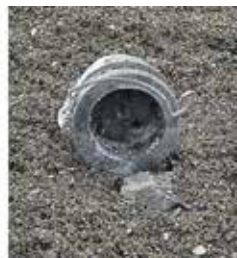
New liner three: in both mortars, the HE burned to deflagration.
