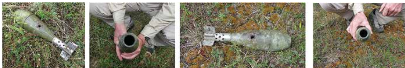
New liner four: an ideal result with all HE burned and no fragmentation.
