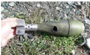
Burned out mortar shell (left) and deflagrated munition (right).
