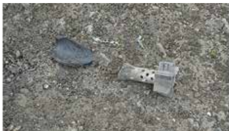
New liner three: in both mortars, the HE burned to deflagration.
